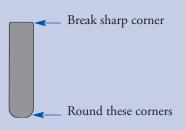
Figure 1 shows the basic terminology of a skew. This shape has evolved over many years and is the shape that experts agree is the most versatile
