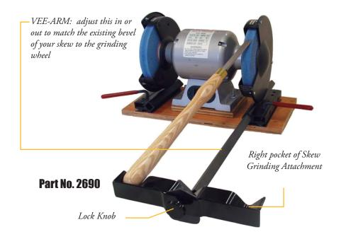
Congratulations on the purchase of your ONEWAY Skew Grinding Attachment. It is used with the ONEWAY Wolverine Grinding Jig. This Skew Grinding Attachment can be used to quickly and easily grind a skew. The unique offset handle position will actually reduce the hollow grind generated and leave a stronger more predictable tool.
