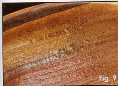
This is a close-up of the same tearout. Notice the surface gaps created by tearing the fibers.
